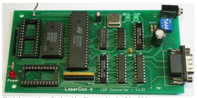
Check that your LaserCon board has Firmware Version 7.0 or higher Set The dip-switches: ON-OFF-OFF Done! Your LaserCon board can now operate with MACH 3.
