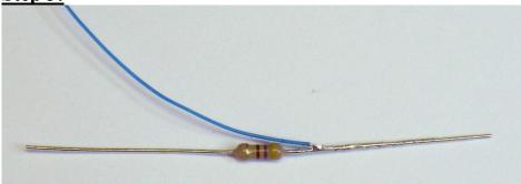
Solder a wire to a 470 ohm resistor.
