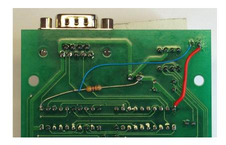
Add a wire from U8 pin-20 (+5V) to the far side of the new 2 pin connector.
