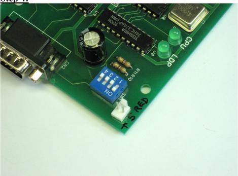
+5 Volts will be supplied to the board through this 2-pin connector. Mark the right side pin to indicate +5V.
