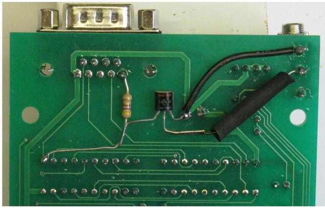
Slip a piece of heat shrink tubing (or black tape) over the resistor, and solder to the middle leg of the transistor.
