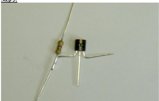
Place the transistor flat side down. Bend legs as shown. Solder resistor as shown.
