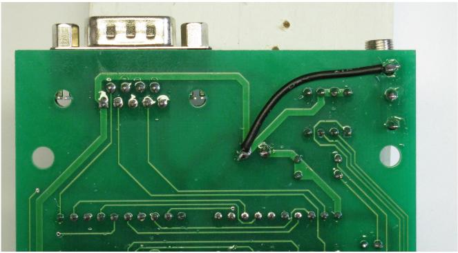
Solder in a ground wire to the negative side of capacitor C1
