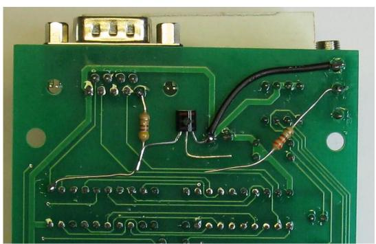
Solder one end of the second resistor to the middle terminal of the Jack.
